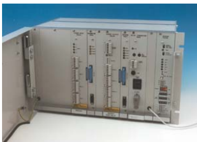
Telecode TDM 19" subrack for Electricity Distribution inter-tripping systems
