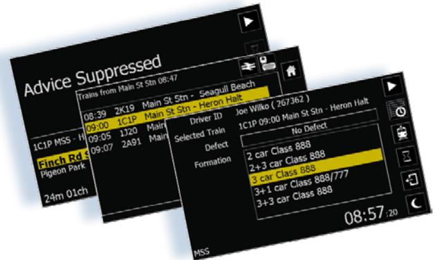
With the Schedule Advisory System, the driver now has more control over achieving on-time arrival of the train. The train's location is continuously compared with an optimum route profile that is engineered to save energy by utilising unused recovery time in the timetable.
