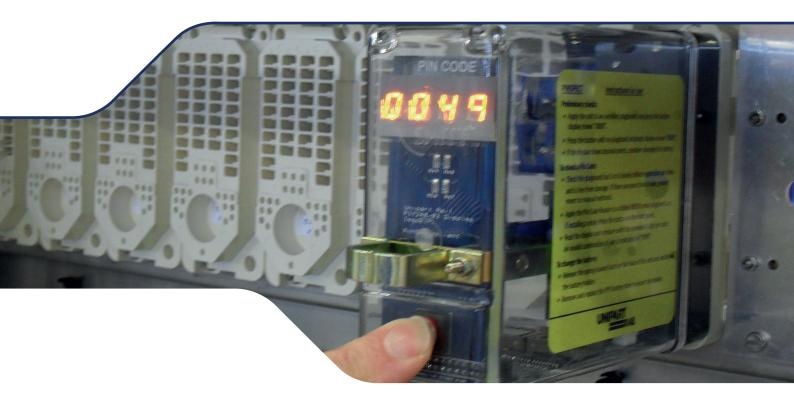
A device to identify or check the drilled holes in a BR930 series plugboard, prior to installation of a new or replacement relay in a location case, REB or relay room.
