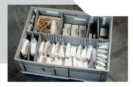
The FlexiKitting solution provided by Unipart Rail creates a seamless supply of materials to ensure that the delivery of maintained vehicles is kept on schedule. All of the parts are placed in re-usable boxes that are divided into sections for each component for ease of identification by the fitter.
