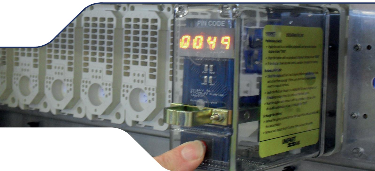
A device to identify or check the drilled holes in a BR930 series plugboard, prior to installation of a new or replacement relay in a location case, REB or relay room.
