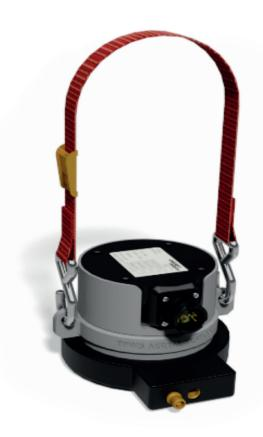
The TPWS Hand Held Signal Generator is programmed to transmit sequences of signal pulses, initialised by the handset controls. Each single pulse consists of a TPWS operating frequency / frequencies, emitted for a specific duration. Time intervals between these different pulses are arranged to simulate TPWS Trackside Sub-System signal profiles.
