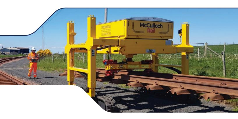
Variable track width allowing access and use in narrow environments
