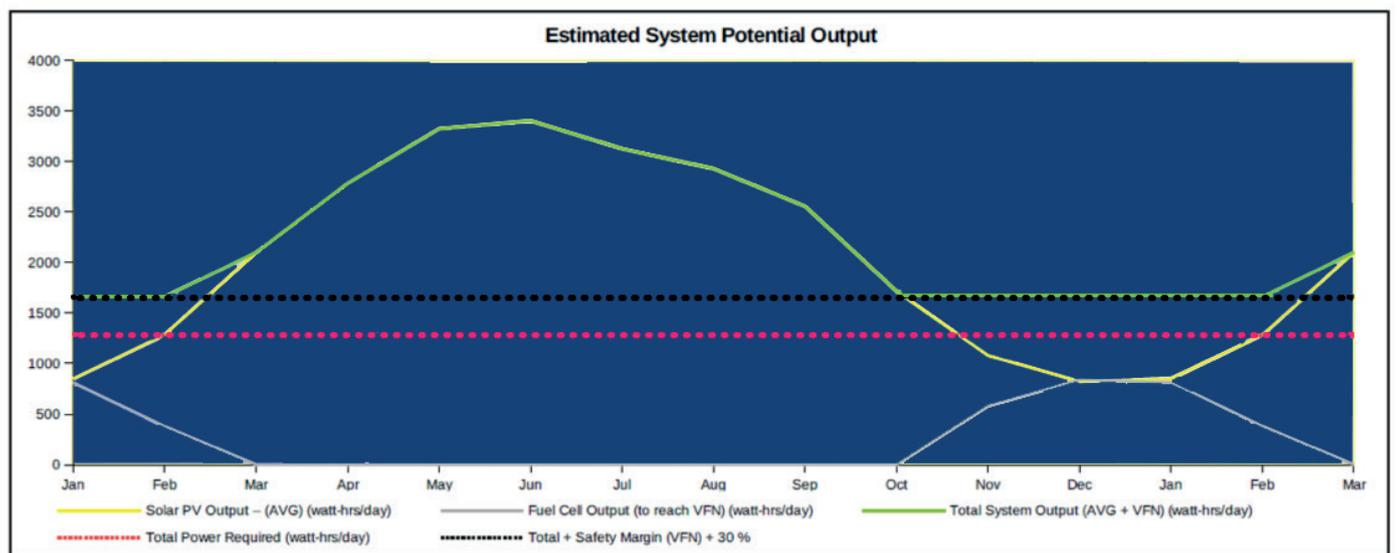
The system design includes a Safety Margin of 30% above the average Meteorological weather data. (as sampled over a 10 year period for the specific site location of the installation).
