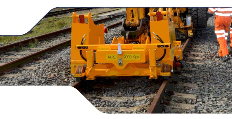
Remove clips at up to 2.5 miles of track per hour Simple, safe, efficient and proven technology Automatic system to prevent sleeper damage Fully approved by Network Rail
