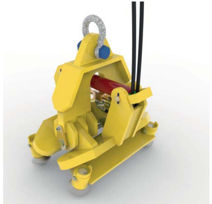
Example: RT10-01-01 Thimble with no pressure control valve or stillage
