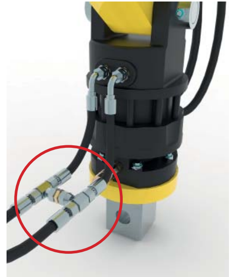
Rotator hoses are connected together using a small bore fitting to dampen out shock loadings
